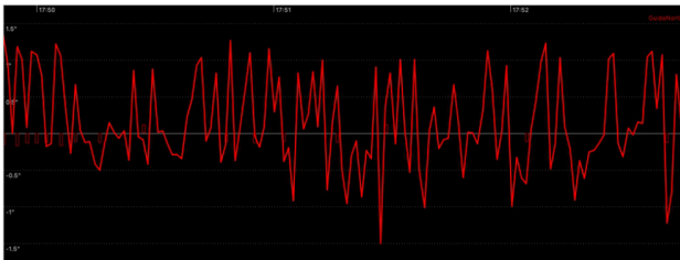
The DEC trace, using Z-filter, for a well PA aligned mount. Note that the correction pulses are few and far between, indicating that the guiding commands are only issued when really needed.
